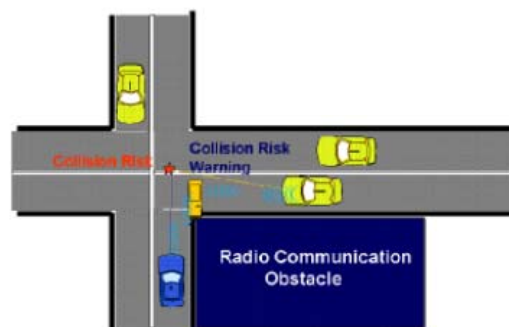
Figure 11 – Road Crossing collision detection
